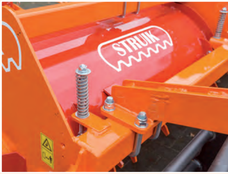
Self-cleaning top cover on springs
